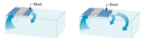
When the required duct is short, the static pressure can be set lower. When the required duct is long, the static pressure can be set higher.
