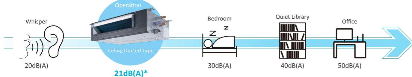
Note: The data was measured in an anechoic chamber, only the DC ceiling ducted type (AVE-05HJFDL) in low noise mode achieves 21dB.
