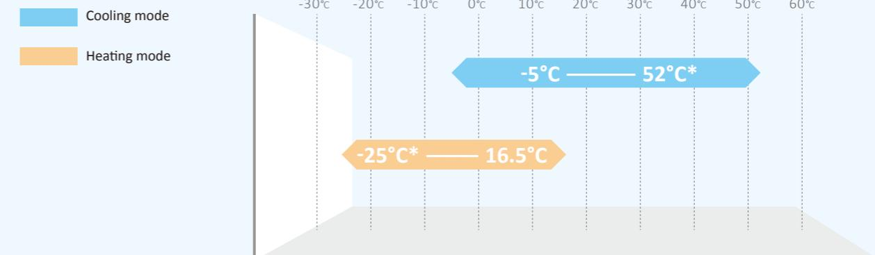
Note: When the temperature is in 48°C~52°C and -20°C~-25°C, the module is in intermittent operation.
